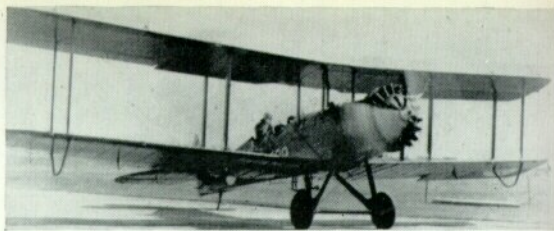
One of the D.H.9s used by Holland, fitted with a Wright Whirlwind engine.
