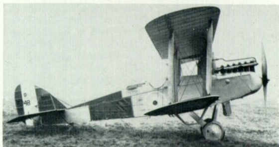
C6078 at Farnborough, fitted with the first Napier Lion engine. When this photograph was taken hot-air pipes and muffs had been added in order to heat the carburettor air intakes. (Photo: Imperial War Museum MH3514)
